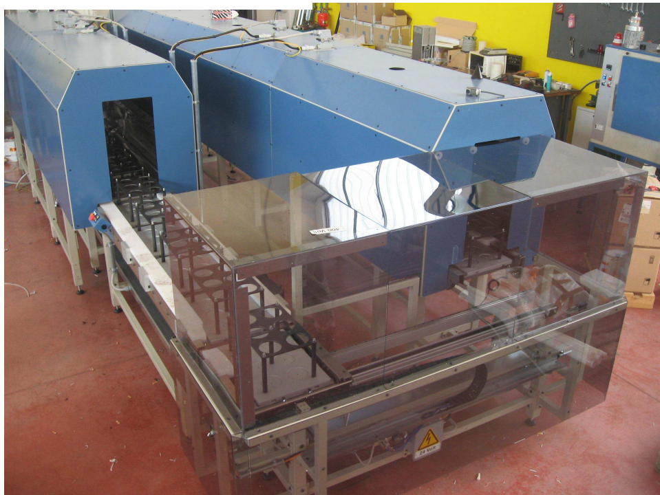
Automatic line with vacuum chamber for encapsulation of motors IP66. This line produces 50 motors/hour.
