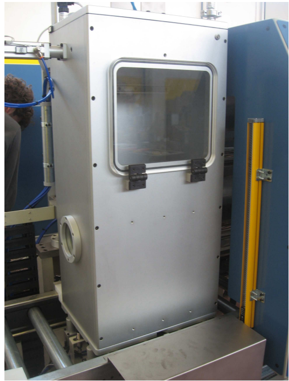
Vacuum chamber with X-Y axes system. This line produces 60 motors/hour.
