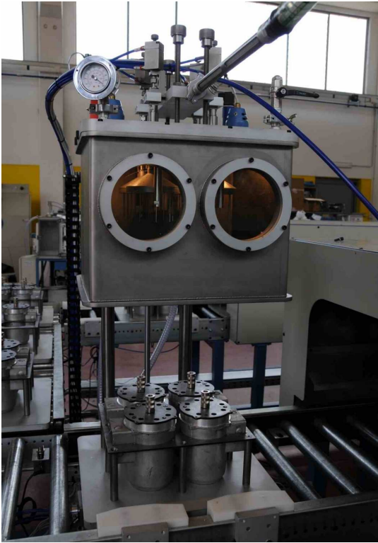
Automatic line with vacuum chamber for encapsulation of motors IP66. This line produces 50 motors/hour.
